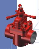
4-1/16" 1000psi Conform to API flange dimensions and pressure classes. Offered with threaded, flanged or weld connections. An economical non-rising stem design.
